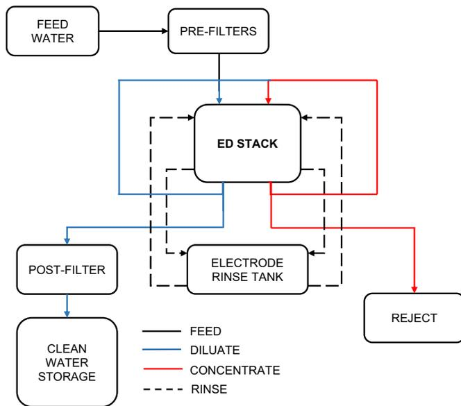
Fig. 3. Flow diagram for continuous ED process.
