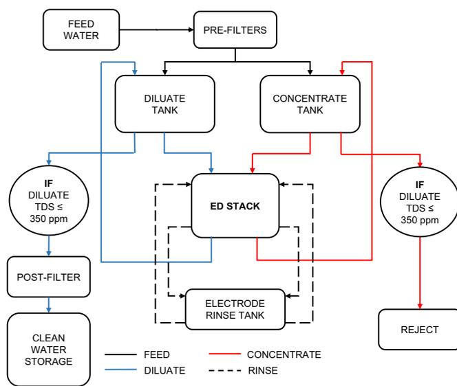
**Fig. 2.** Flow diagram for batch ED process.
