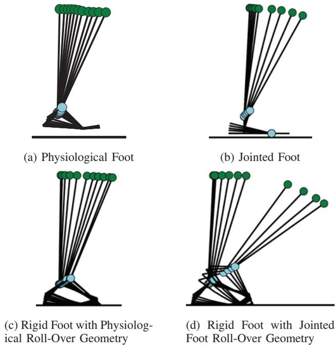
Fig. 6: Comparison of physiological lower leg trajectory from able-bodied gait data (a) with the optimized jointed foot model ( $LLTE = 0.17$ ) (b), a rigid foot with physiological roll-over geometry ( $LLTE = 1.32$ ) (c) and a rigid foot with roll-over geometry exactly matching the roll-over geometry of the jointed foot ( $LLTE = 2.09$ ) (d).
