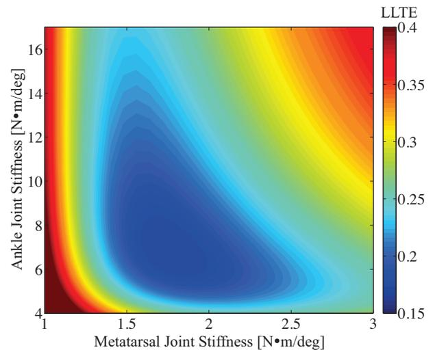
Fig. 5: *LLTE* values calculated for the jointed foot model in Fig. 3 over a range of metatarsal and ankle joint stiffnesses. The optimal stiffness values are those which produce the minimum *LLTE*. In this case the minimum *LLTE* value is 0.17 for ankle stiffness of 6.7 N·m/deg and metatarsal stiffness of 1.8 N·m/deg.
