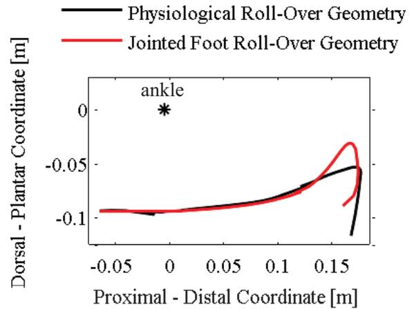
Fig. 8: A comparison of the roll-over geometry of the conceptual jointed foot model optimized for lower leg trajectory and the physiological roll-over geometry ( $R^2 = 0.52$ ).
