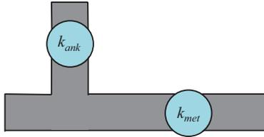
Fig. 3: Analytical model of prosthetic foot consisting of rotating joints at the ankle and metatarsal with constant rotational stiffnesses,  $k_{ank}$  and  $k_{met}$ , respectively.
